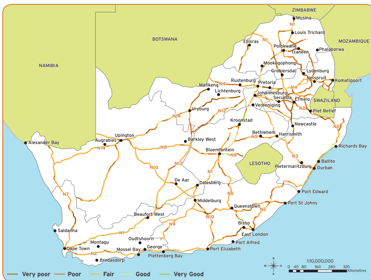
Figure 27: Visual condition of major road networks of South Africa
