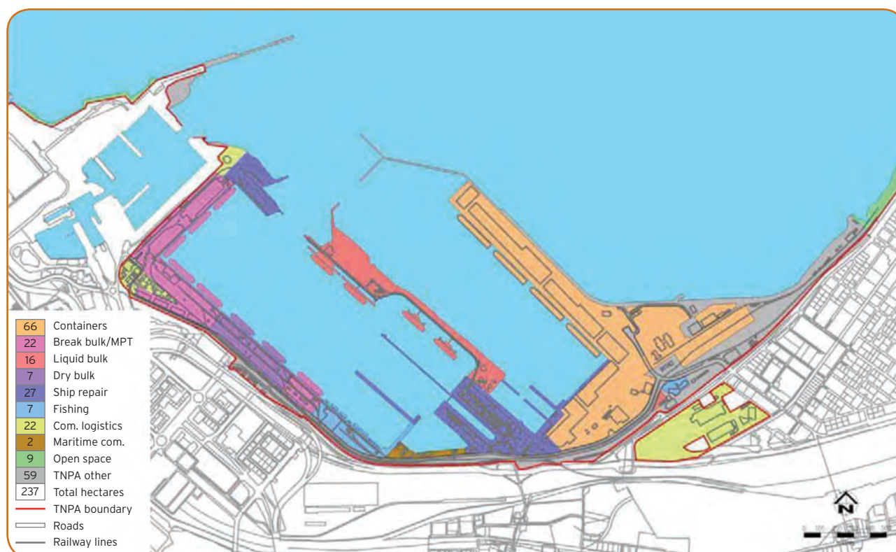
Figure 12: Port of Cape Town, layout and facilities
